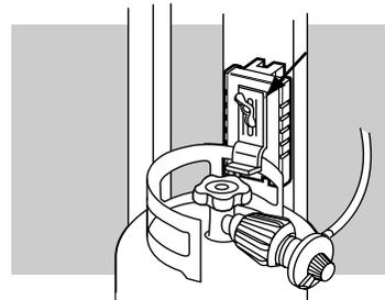
Screw the regulator coupling onto the cylinder valve(1), clockwise, or to the right. Hand tighten only.
