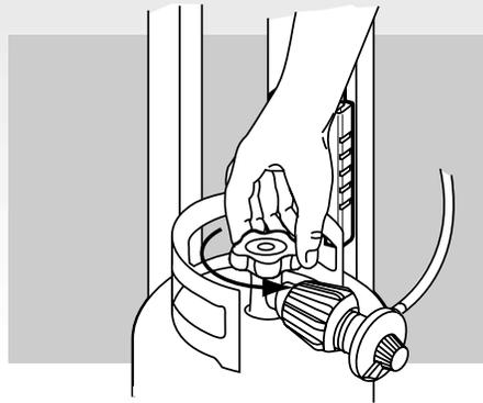
If there is a leak, turn off the gas and tighten the fitting. Turn the gas back on and recheck with the soap and water solution.
