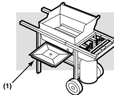
**Put the disposable drip pan into the catch pan.**
